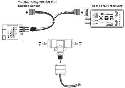
Connect the T-Connector to the pressure measuring head.
